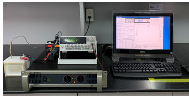
Figure 1. Photograph of the experimental ohmic heating (OH) system
