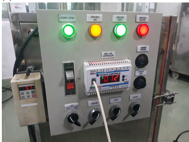
Figure 1. Halogen dryer: (A) the dryer; (B) DDC-C46 controller
