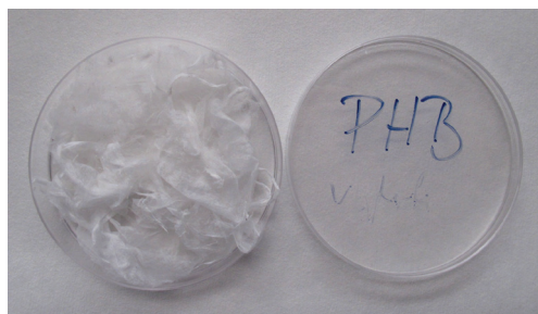
Figure 1. 3D fluffy structure of PHB fibres
